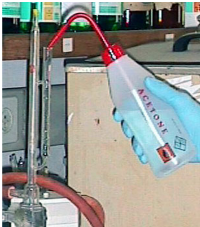
Insert the tube completely and Wash the inside of the tube
