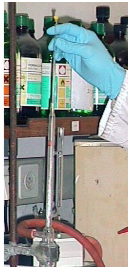
Place cap on the bottom of the NMR tube and insert the tube
