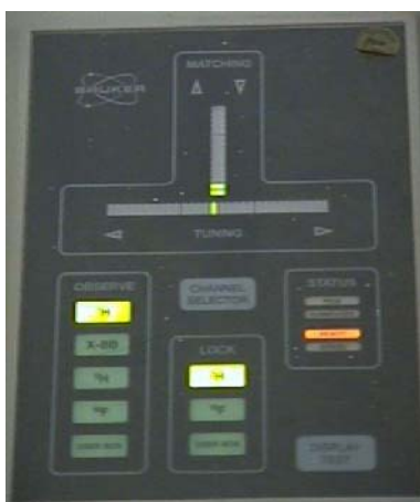
Fig. 27. The display on top of the preamplifiers showing that the probe is tuned and matched
