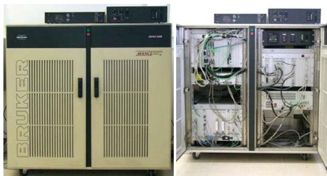
Figure 2. The console of the 400 MHz spectrometer with the doors closed on the left and open on the right
