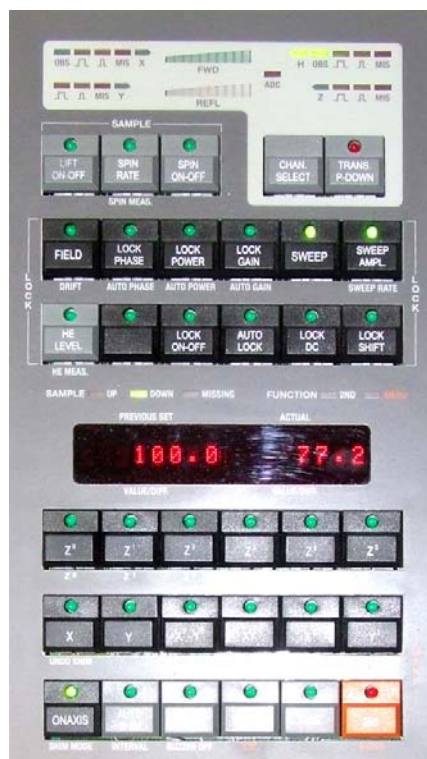
Figure 17. The control panel of the 500 MHz spectrometer for sample handling and magnet control as seen from above
