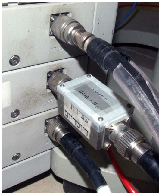
Figure 64. The 2H stop filter connected to the X channel of the preamplifiers
