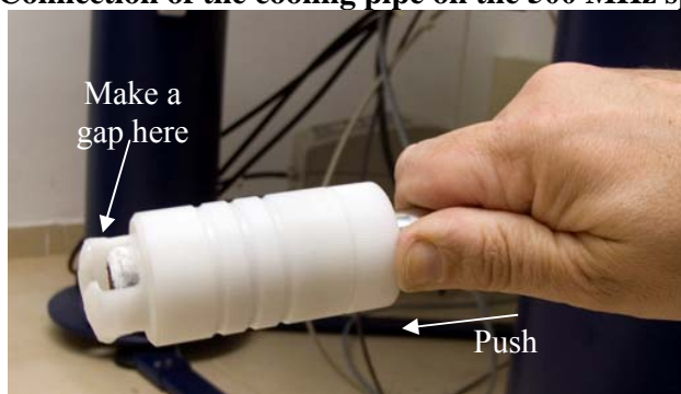
Figure 45. The cooling pipe connected to the probe of the 500 MHz spectrometer
