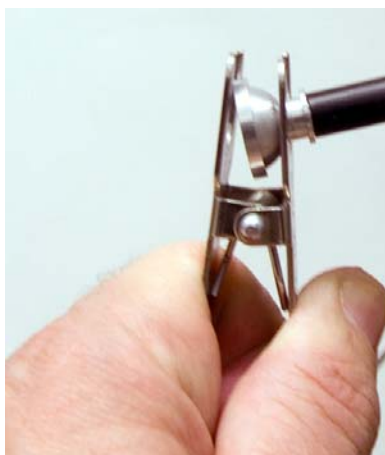
Figure 41. Opening the air hose clip
