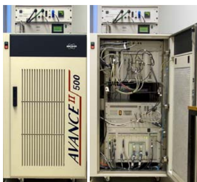
Figure 4. The console of the 500 MHz spectrometer with the door closed on the left and open on the right
