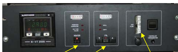
Heater button Cooler button Flow gauge Read the value at the bottom of the ball
