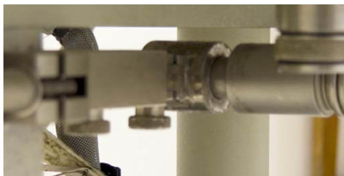
Figure 42. Clamp for the cooling pipe under the magnet
