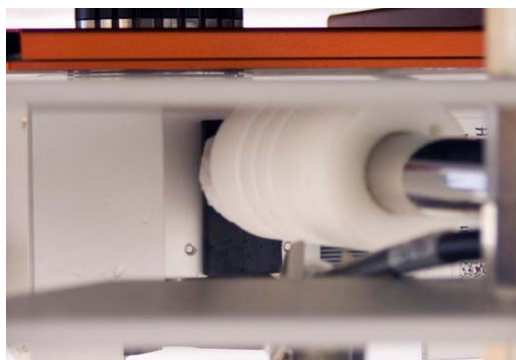
Figure 45. The cooling pipe connected to the probe of the 500 MHz spectrometer
