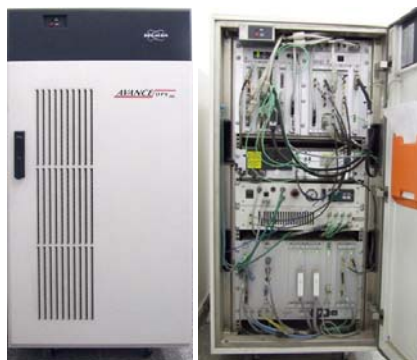
Figure 3. The console of the 200 MHz spectrometer with the door closed on the left and open on the right
