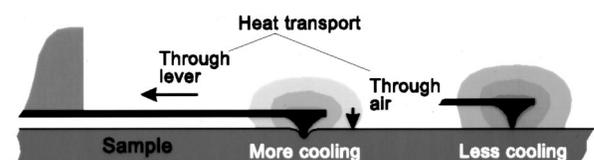
FIG. 3. Principle of AFM thermal sensing. The tip of the heater cantilever is continuously heated by a direct current power supply.
