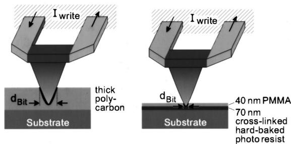
FIG. 1. (a) Previous storage medium consisting of a bulk polycarbonate layer. (b) For smaller bit sizes, a new storage medium consisting of a thin writable PMMA layer on top of a Si substrate with a crosslinked film of photoresist in between is used.
