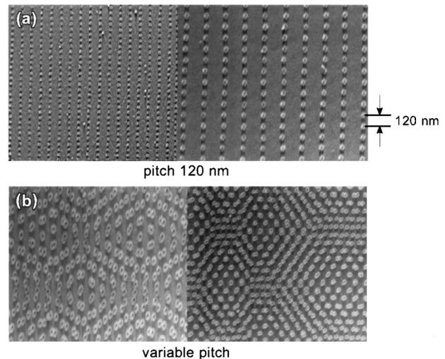
FIG. 2. (a) Series of 40 nm data pits formed in a uniform array, demonstrating reliable thermal writing. (b) Different arrangement of data pits, with some pits written virtually next to each other with no merging. This results in bit areal densities of  $\approx 400$  Gbit/in.<sup>2</sup>. All images obtained by the thermal readback technique.
