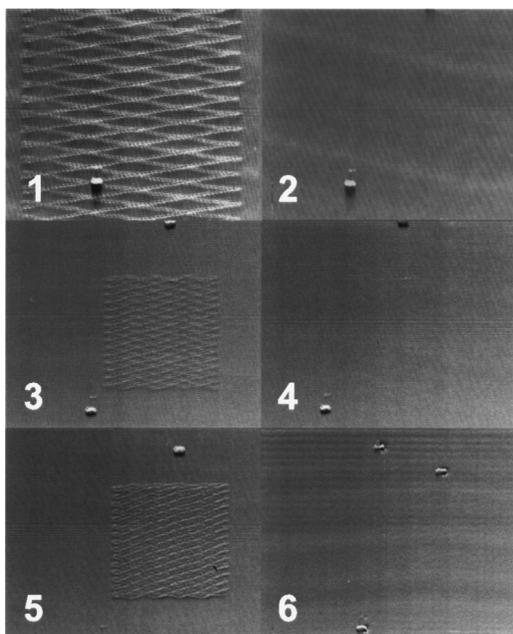
FIG. 4. AFM image of thin PMMA layer demonstrating three erasing/rewriting cycles.
