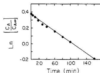
**Figure 5.** Deactivation of the NEt<sub>3</sub>BzBr catalyst presented by plot of a  $\ln \ln (C_A/C_{A0})$  vs. time. Data from Figure 4.
