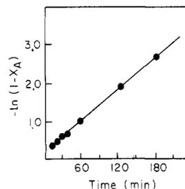
**Figure 3.** First-order kinetics of the elimination of (1-chloroethyl)benzene in presence of NBu<sub>4</sub>-HSO<sub>4</sub>. Reaction conditions: 70.9 mmol of substrate, 35 mL of 50% NaOH solution, 3.55 mmol of TBA-HSO<sub>4</sub>; 75 °C; stirring at 1000 rpm.
