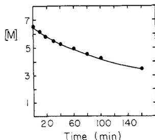
**Figure 4.** Reaction profile of the elimination of HBr from (2-bromoethyl)benzene with TEBA-Br catalyst. Reaction conditions: 66.5 mmol of substrate, 840 mg of toluene, 35 mL of 50% NaOH, 0.665 mmol of TEBA-Br; 75 °C; stirring at 1000 rpm.
