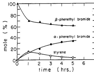
Figure 1. Elimination and isomerization of (2-bromoethyl)benzene in presence of 5 mol % NBu<sub>4</sub>Br at 155 °C.
