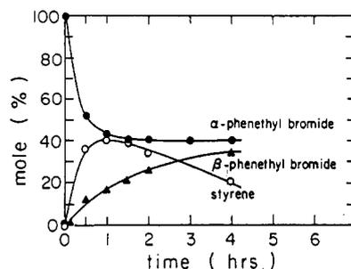
Figure 2. Elimination and isomerization of (1-bromoethyl)benzene in presence of 5 mol % NBu<sub>4</sub>Br at 155 °C.
