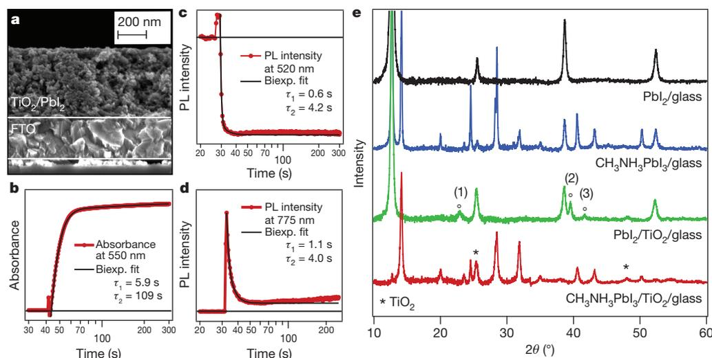
**Figure 1 | Transformation of  $\text{PbI}_2$  into  $\text{CH}_3\text{NH}_3\text{PbI}_3$  within the nanopores of a mesoscopic  $\text{TiO}_2$  film.** **a**, Cross-sectional SEM of a mesoporous  $\text{TiO}_2$  film infiltrated with  $\text{PbI}_2$ . FTO, fluorine-doped tin oxide. **b**, Change in absorbance at 550 nm of such a film monitored during the transformation. **c**, Change in photoluminescence (PL) intensity at 520 nm monitored during the
