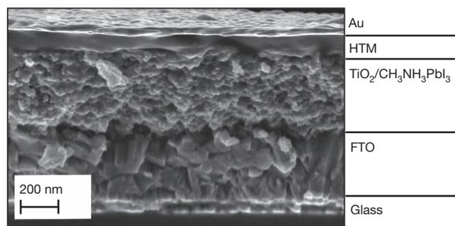
**Figure 2** | Cross-sectional SEM of a complete photovoltaic device. Note that the thin  $\text{TiO}_2$  compact layer present between the FTO and the mesoscopic composite is not resolved in the SEM image.
